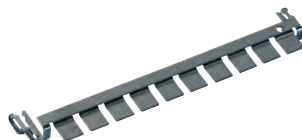
LSA 2/10-ES (Art.No. 24 01 33) Pluggable grounding rail: For 10DA connection modules serving as connection between LSA backmount frame and 1 DA surge voltage (+surge current) protection connector Installation: Plug into front connection modules, bonding to ground via LSA backmount frame
