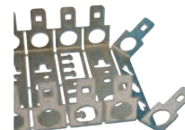
LSA 2/10-MW10-25/22 (Art.No.24 01 10) LSA backmount frame 10 x 10DA (modular) stainless metal. Plug space for 10 pcs of LSA 2/10 10DA connection modules 25 mm grid / depth 22 mm, easily detachable upon individual requirements, available up to a size of 78 connection modules.
